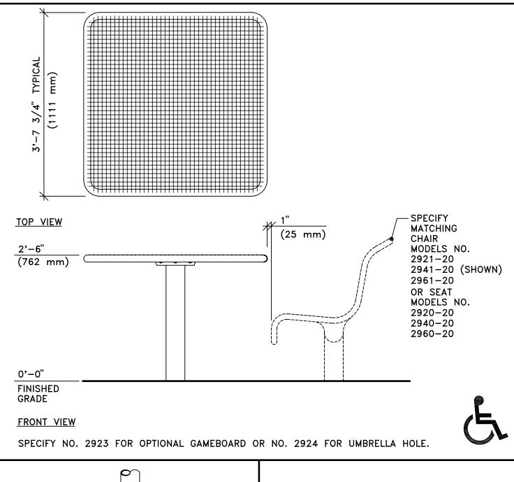
0'-0" FINISHED GRADE NOTE: (ab CONCRETE FOOTING AND NO. 4 REBAR (BY OTHERS) PER LOCAL SOIL CONDITIONS, CONSULT PROJECT ENGINEER FOR -(1'-6") -(457 mm) EXACT REQUIREMENTS.
